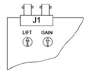
**Default Position.** For shorter cable lengths, turn the relevant control anticlockwise until the required picture quality is obtained. For longer cable lengths, turn the relevant control clockwise until the required picture clarity is obtained.
